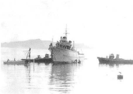
A "TON" CLASS COASTAL MINESWEEPER OF THE S A NAVY (POSSIBLY SAS KIMBERLEY) BEING POSITIONED ON THE CRADLE PRIOR TO BEING HAULED UP ON THE WEST DOCKYARD SLIPWAY BUILT BY DE PASS, SPENCE & Co. - Photo : Simon's Town Museum
